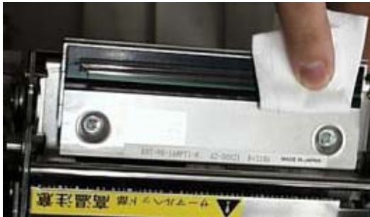
Wipe the heat element component of the thermal head several times only in one direction
