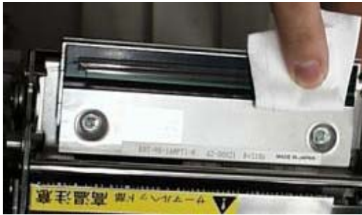
Wipe the heat element component of the thermal head several times only in one direction
