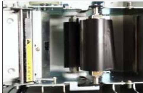
Put the winding ink ribbon on the V notch of Upper cover to see the thermal head surface correctly.
