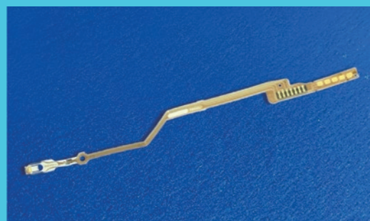
Thin-film metal base board (CISFLEX™)
